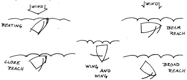
A beam reach is a point of sail with the wind perpendicular to the center line of the boat. To trim sail properly, steer your desired course and let the sails out until they luff (flutter) slighty (watch along the mast for the mainsail and along the luff pole for the jib) and then pull them in again to a point at which the luffing stops. You want the sails just on the verge of luffing. If the tiller is hard to handle, or the boat wants to swing into the wind, your sails are probably in too far.
