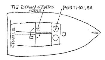
When trailering a one piece mast, this cradle can be used to keep all of the spars secure. The cradle is strapped to the boat with a line that goes underneath the hull. The mast is placed in the yoke and tied down with a line going through the
