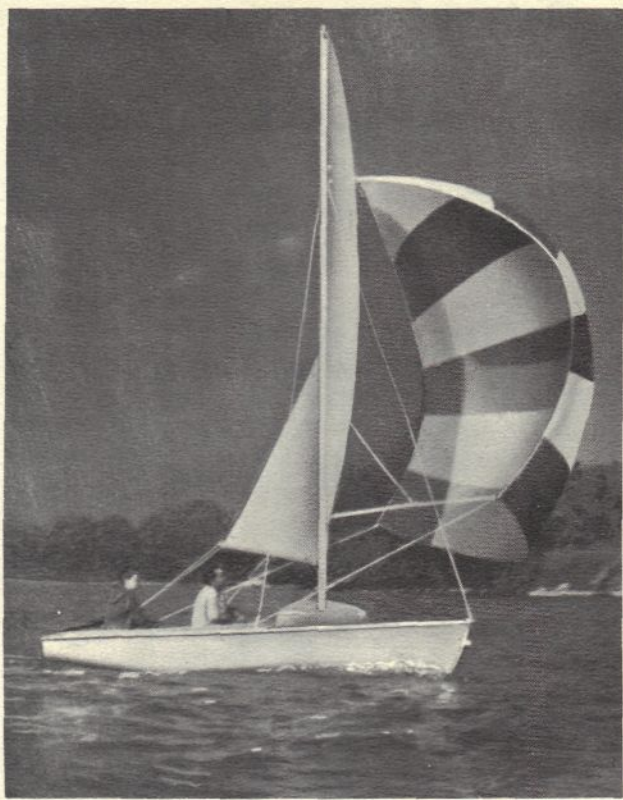
"More sail - more speed"— the spinnaker provides the thrill of racing with an ease of handling. Spinnaker area 130 sq. ft.
